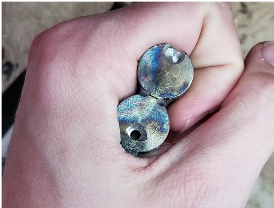
Figure 5: Top of firing pin hole rounded out. Try not to remove more material than this.
