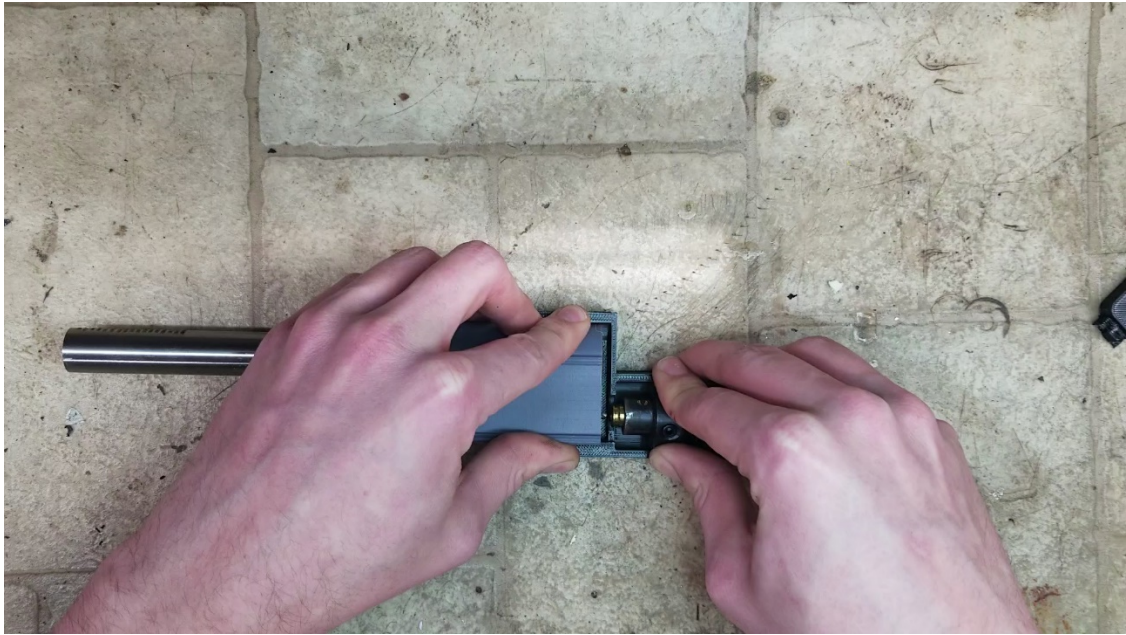
Checking firing pin alignment
