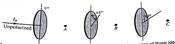
2c. A beam of unpolarized light of intensity lopasses through a series of three ideal polarizing filters with their polarizing directions turned to the angles shown above.
