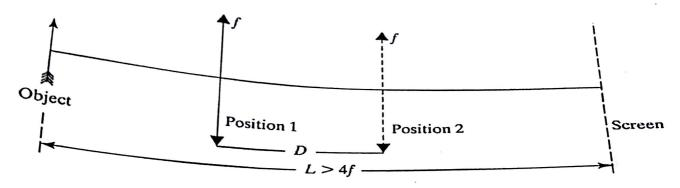
3b. 8(pt) Bessel's method for finding the focal length of a lens is described in the figure above. The object and screen are at a fixed distance L greater than 4 times the unknown focal length. The single lens is moved between the object and the screen. The image is in focus on the screen for two different positions of the lens separated by distance D. What is the focal length of the lens in terms of L and D?
