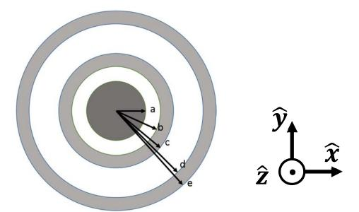
**5) 15 pts** The figure above shows a cross-section through a tri-axial cable that extends infinitely far into and out of the page. The center conductor (from radius 0 to a) carries current  $I_1 = 3 I \hat{\mathbf{z}}$ . The middle conductor (from radius b to c) carries current  $I_2 = -5 I \hat{\mathbf{z}}$ . The outer conductor (from radius d to e) carries current  $I_3 = 2 I \hat{\mathbf{z}}$ . What is the magnetic field  $\mathbf{B}(r)$  in the region with radius r between d and e?
