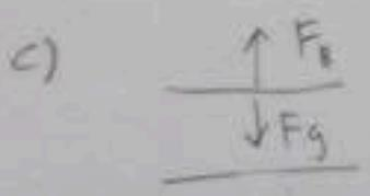
top wire needs magnetic force upward to balance out gravity
