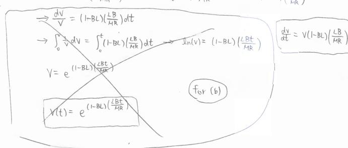
(b) Explicitly solve this first-order differential equation by separating variables to obtain an expression for the speed as a function of the time, t. Be sure to use the appropriate initial condition, as well as to express the result in terms of the given quantities. [12]
