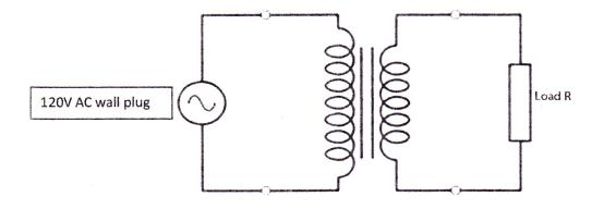
I hook up a neon sign transformer to a load with resistance  $R_{load}$  and plug the primary into a wall outlet. The transformer primary is rated 120 V and the secondary is rated 12,000 V.
