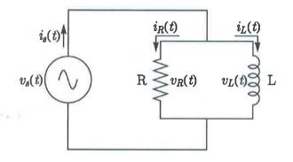
(a) Use Kirchhoff's circuit law for currents to obtain an expression relating the current from the source  $i_s(t)$  to currents through the resistor and the inductor. Use Kirchhoff's circuit law for voltages to obtain expressions relating the voltage from the source  $v_s(t)$  to voltages across the resistor and across the inductor.
