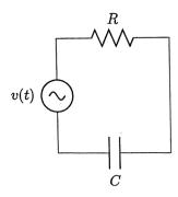
(a) With the aid of a phasor diagram, or otherwise, obtain the impedance and phase angle of the circuit in terms of  $\omega$ , R and C.
