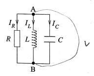
The current through the capacitor can be written in terms of V and C using the equation V = q/C, so that
