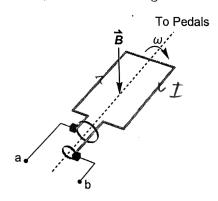
(a) If Ryan is pedalling at a constant angular velocity  $\omega$ , find an expression for the induced emf  $\mathcal{E}(t)$  around the loop as a function of time. [Assume the vector area of the loop  $\vec{\mathbf{A}}$  is parallel to  $\vec{\mathbf{B}}$  at t = 0. . Wt = 90°
