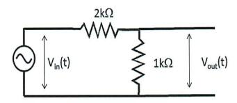
Design a simple circuit that instead that "blocks" signals with frequencies 60 Hz or less by making the amplitude of  $V_{out}(t)$  only 1% of the amplitude of  $V_{in}(t)$ . Your circuit should still pass signals with very high frequencies (for example >1 kHz or more) with at least 95% of the input amplitude. This is an example of a very common circuit used to reduce noise
