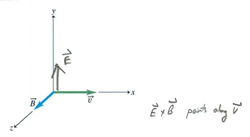
the direction of propagation is shown as  $\mathbf{v}$ . The direction of the magnetic field in the is shown as  $\mathbf{B}$ . On the figure above, draw the direction of the electric field  $\mathbf{E}$  at the origin.
