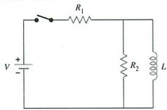
Suppose the battery has a 1.5 Volt EMF and that resistor  $R_1$ =1  $k\Omega$  and  $R_2$ =2  $k\Omega$ . A long time after the switch is closed, what is the current through resistor  $R_2$ ?
