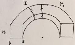
A second toroidal solenoid with inner radius c (< a), outer radius d (> b), height  $h_2$  (>  $h_{1)}$ , and  $N_2$  turns that carry a current  $I_2$  concentrically surrounds the first solenoid as shown in cross-section.
