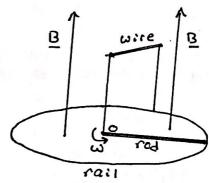
Recall that the moment of inertia of the rod about the z- axis is  $m L^2/3$ , and that the differential torque is  $d\tau = r x dF$ .
