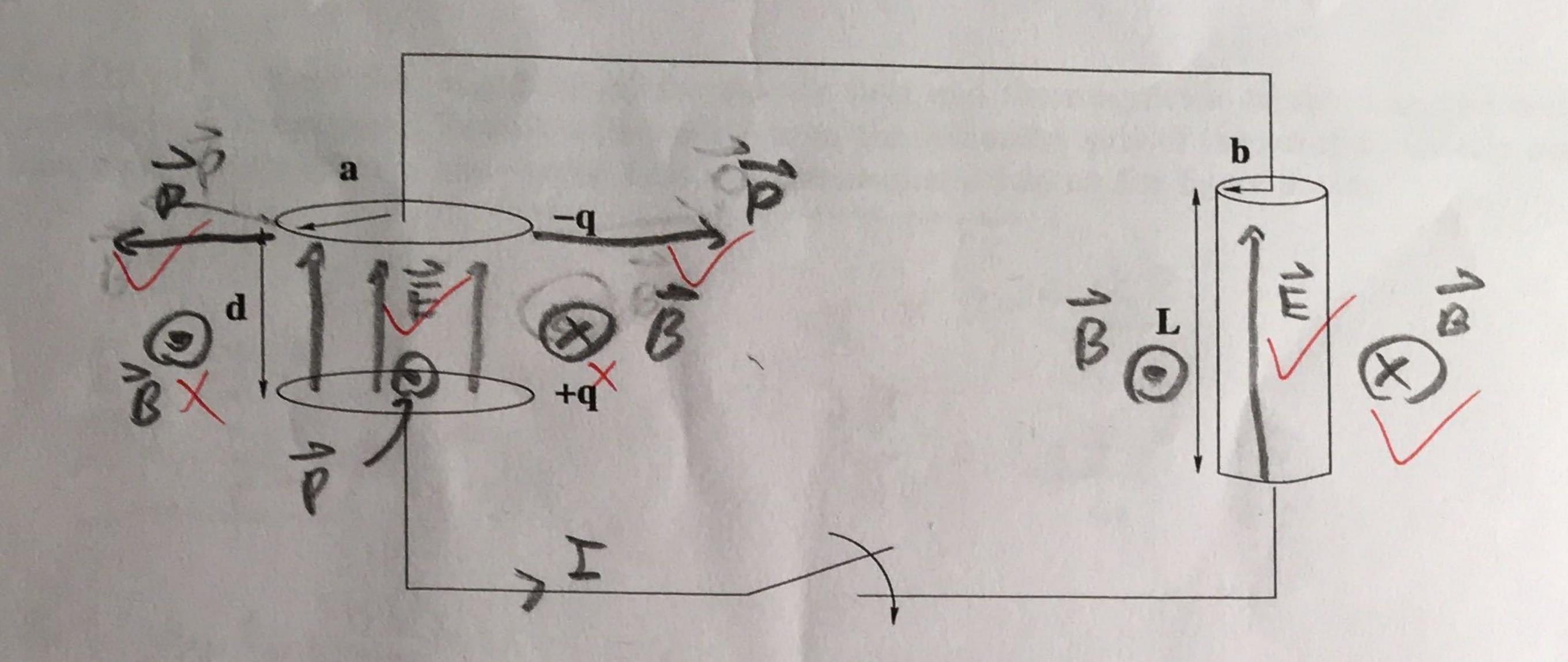
1) A circular parallel-plate capacitor of plate radius a and plate separation d is connected across a cylindrical resistor of radius b and length L At the instant under consideration, the capacitor has a charge q, with the polarity given in the figure.
