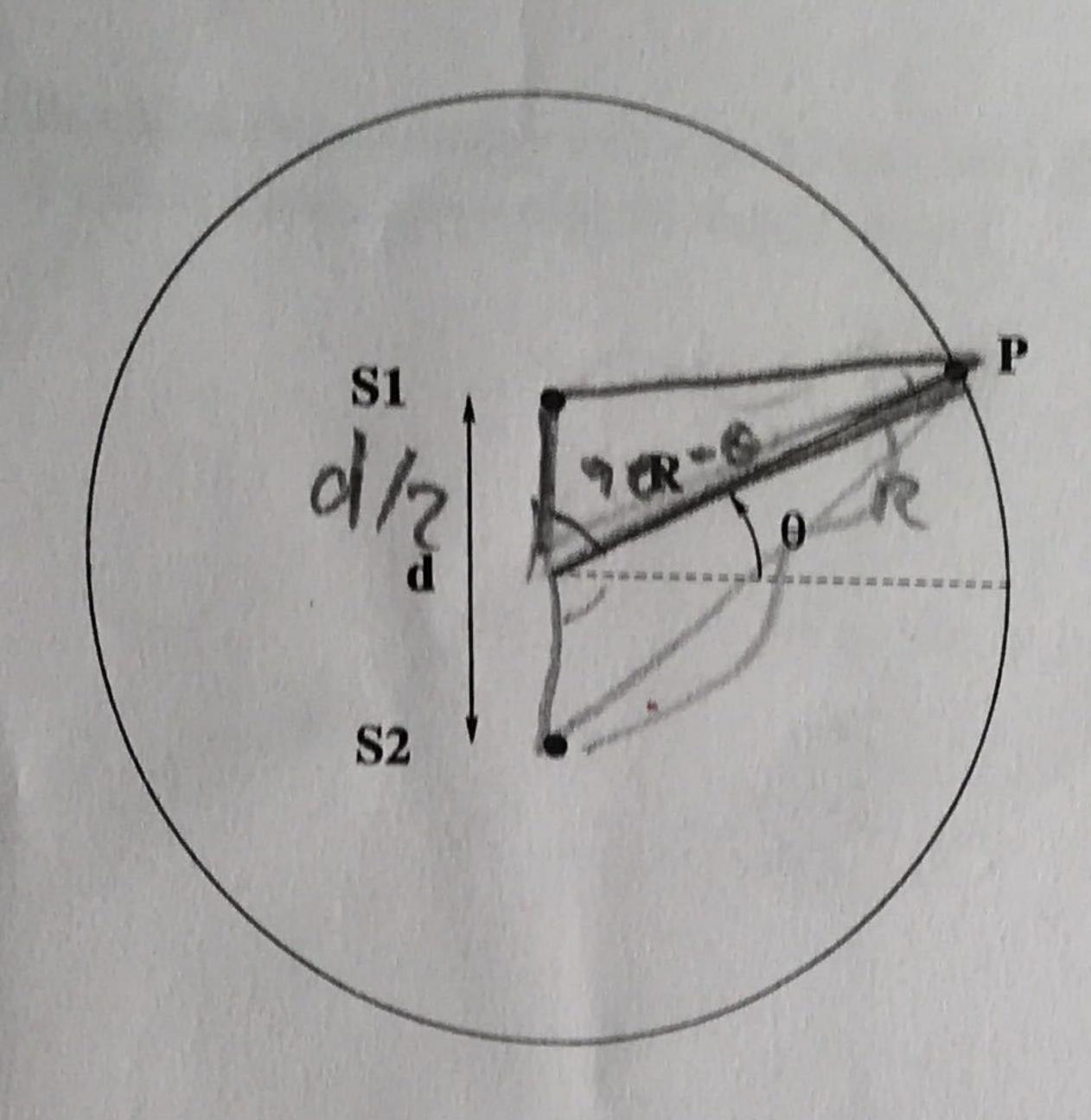
3) It is possible to use interference to create antenna arrays that preferentially radiate radio-frequency energy along preferred directions ("lobes") in the azimuth.
