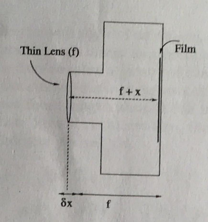
2) The important parts of the camera shown above are the film and the converging lens of focal length f. The distance between the lens and the film is given by f + x, where x can be adjusted to any value between 0 and  $\delta x = f/10$  to bring the subject to be photographed into focus.
