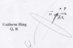
2) A uniform circular ring of charge Q and radius R rotates around its longitudinal symmetry axis with an angular velocity  $\vec{\omega}$ , as shown.
