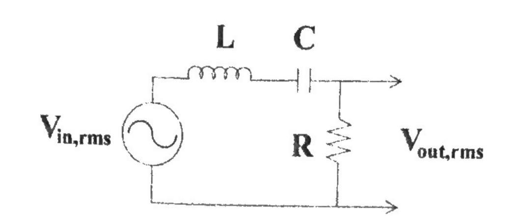
Filters are classified by the frequency-range of the signals they deliver to their output. High-pass and low-pass filters preferentially pass high- and low-frequency signals, respectively. Band-pass filters preferentially pass signals that have frequencies within some range (or band') of frequencies. Notch filters actually remove signals whose frequencies lie within some range of frequencies.
