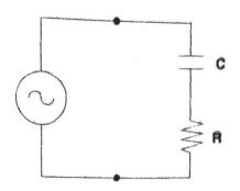
3) An capacitor (C) and a resistor (R) are connected in series across a source of alternating EMF  $(\xi(t) = \xi_{max} \cos(\omega t))$ . You may do the following calculations in complex space, but keep in mind, the final answers must all be real.
