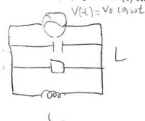
$$V = I \neq 1, Z = \sqrt{R^{2} + (\omega_{L} - \frac{1}{\omega_{C}})^{2}} \quad V_{R} = IR \quad V_{L} = I\omega_{L}, \quad V_{L} = i\omega_{L}$$
