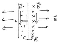
A dipole antenna is constructed from two pieces of wire, fed in the center (you can probably ignore that), that add up to a total length L, as shown. At the moment under consideration, an electric current I flows upward through the dipole and electromagnetic energy radiates radially outward from the dipole.
