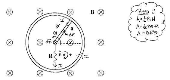
A conducting rod of length a extends from a central conducting hub to a conducting ring of radius a. It rotates around the conducting hub with an angular speed  $\omega$ , in the plane of the page, as shown. The conducting hub is joined to the conducting ring by a resistor of resistance R. The whole apparatus is immersed in a uniform magnetic field  $\mathcal{I}$  which points into the page.
