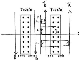
A pair of large, wide current sheets of finite thickness b=a are positioned parallel to the x, y-plane, symmetric about the origin, as shown. Each carries a current described by the density  $\vec{J} = J(-\hat{x})$  out of the page.
