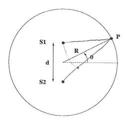
3) It is possible to use interference to create antenna arrays that preferentially radiate radio-frequency energy along preferred directions ("lobes") in the azimuth.
