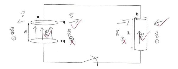
1) A circular parallel-plate capacitor of plate radius a and plate separation d is connected across a cylindrical resistor of radius b and length L At the instant under consideration, the capacitor has a charge q, with the polarity given in the figure.
