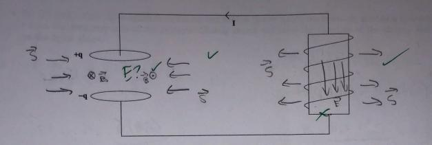
A circular parallel-plate capacitor of plate area A and plate separation d is connected across a solenoidal inductor of radius a, length x and n turns per unit length. At the instant under consideration, the capacitor has a charge q (polarity shown above), and a current I is flowing through the circuit in the direction shown. We do not know the instantaneous rate at which the current is changing, but it may be possible to infer that from the other information we know.
