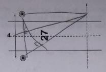
A simple navigation system consists of two radio-frequency antennas fed in-phase with a signal of wavelength  $\lambda$ . The antennas lie along a line that runs perpendicular to the runway, they are equidistant from the center of the runway, and they are separated by a distance d. Incoming aircraft are supposed to locate the central maximum generated by the resultant signal and follow it to a safe landing on the airstrip below.
