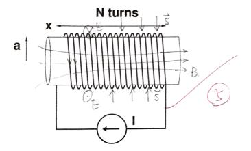
An inductor is wound over a cylindrical form of radius a and has N turns evenly spaced over a length x as shown. It is connected across a source that supplies a constant current I in the direction shown.
