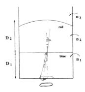
A beaker contains two layers of fluid. The blue fluid that sits on the bottom has an index of refraction  $n_1$ and fills the beaker to a height  $D_1$ . The red fluid on top has an index of refraction  $n_2$  and spans a depth  $D_2$ . The interface between the fluids is flat. The interface between the top fluid and the air above it (of index  $n_3$ ) is curved upward with a radius of curvature of magnitude |R| (Large compared to either value of D, but small enough to be noticeable).
