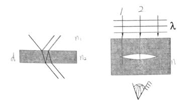
• 3a) (10 points) Monochromatic light strikes a thin film in near-vertical incidence. Using interference principles, show that when the light reflected off the top of the film undergoes constructive interference, the light transmitted through the film undergoes destructive interference, and vis-versa.
