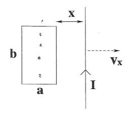
2) In the diagram above, a rectangular conducting loop (dimensions a and b, resistance R) and a long straight wire that carries an electrical current I are both oriented so that they sit in the plane of the page. They will, for the duration of the problem, remain in the plane of the page with the wire carrying an electrical current I parallel to the right side of the conducting loop at a distance x to that side (as shown).
