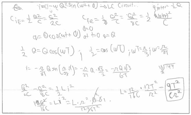
2. An LC circuit consists of a 20.0-mH inductor and a 0.500-F capacitor. If the maximum instantaneous current is 0.100 A, what is the greatest potential difference across the capacitor? (5 pts)
