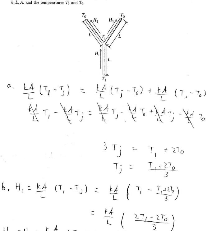
$(T_J - T_O) = \frac{kA}{I} \left( \frac{T_I + 2T_O}{2} - T_O \right) = \frac{kA}{I} \left( \frac{T_I - T_O}{2} \right)$
