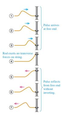
A wave described by the wave function y(x,t) with such a free end must satisfy  $\frac{\partial y}{\partial x} = 0$  at the free end of the string. Find the allowed frequencies of the standing waves on this string in terms of  $\mu$ , T, and/or L.
