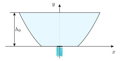
In this problem, we will use Bernoulli's principle and the equation of continuity to calculate the time  $\Delta t$  that it takes for all of the fluid to flow out.
