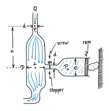
**3.1**. Suppose that the clamp is unscrewed and the stopper is free to move. Find an expression in terms of the given variables for the force exerted by the ram on whatever it's crushing in this circumstance.
