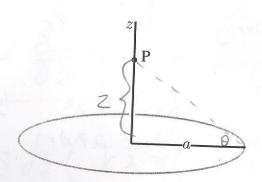
(a.) (10) Find an expression for the electric potential (voltage) at point P, where the potential is chosen to be zero at infinity.
