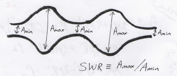
Therefore a very important quantity in engineering and physics is the "standing wave ratio" or SWR which is defined as SWR= $A_{max}/A_{min}$ . Suppose the reflected wave is in phase and has 50% of the incident amplitude. Find the ratio of the envelopes between the places where a node and an antinode would have been if the reflection had been 100% and in phase.
