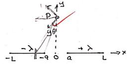
(5) b. If y >> a , and y >> L, show that the magnitude of the electric field is approximately given by  $\left|\underline{E}\right| \approx \frac{\lambda(L^2 - a^2)}{4\pi\epsilon_0 \, y^3}$
