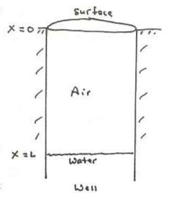
b) at x=0,  $\delta P(0,t) = 0$  since pressure is at a node when the and y(0,t) is at a maximum artificity of at a node when blocked at x=L,  $\gamma(L,t) = 0$  since displacement is at a node when blocked and  $\delta P(L,t)$  is at a maximum (also means (also mea
