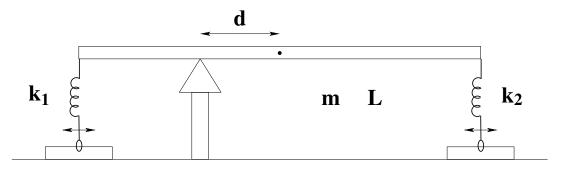
Quiz 1) A uniform rod of mass m and length L pivots around a point located a distance d from its center. On the ends are mounted springs of constants  $k_1$  and  $k_2$ , both of which are cut so that they are unstretched when the rod is horizontal. The bottom of each spring is mounted on a frictionless rail so that the springs remain vertically-oriented when the rod is displaced from a horizontal position.
