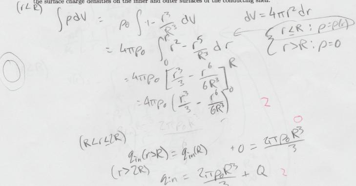
• 3b) (10 points) Find the electric field as a function of the radial distance from the center of the charge distribution (r) for all values of r.
