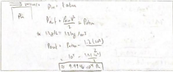
d) At what threshold wind speed will the force on the roof be large enough so that it flies away?
