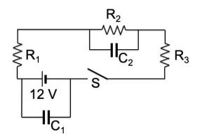
a. The switch is initially open. What are the charges on  $C_1$  and  $C_2$ ? [2 points]
