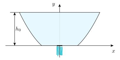
In this problem, we will use Bernoulli's principle and the equation of continuity to calculate the time  $\Delta t$  that it takes for all of the fluid to flow out.
