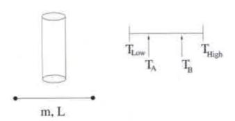
In the apparatus shown, the string (fixed at both ends and driven in its fundamental mode) is used to search for resonant frequencies in the neighboring tube. As the tension in the string is varied from  $T_{low}$  to  $T_{high}$ , the tube is found to resonate at precisely two settings:  $T_A$  and  $T_B$ . For the following, you may assume that the string has a mass m and length L, and you may take the speed of sound in air to be  $v_{snd}$ .
