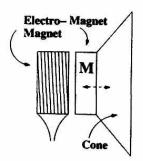
The diagram above shows a very simple loudspeaker. The main part consists of a magnet (mass M) attached to a flexible cone. The speaker is designed so that, in proper use, as the magnet is displaced slightly (left or right) from it's equilibrium position, the cone will push or pull on it with a linear restoring force.
