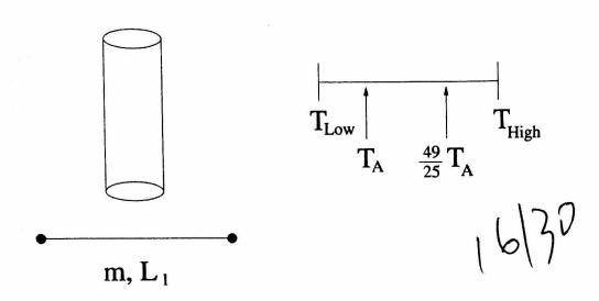
In the apparatus shown, the string (fixed at both ends and driven in its fundamental mode) is used to search for resonant frequencies in the neighboring tube. As the tension in the string is varied from  $T_{low}$  to  $T_{high}$ , the tube is found to resonate at precisely two settings:  $T_A$  and  $\frac{49}{25}T_A$ . For the following, you may assume that the string has a mass m and length  $L_1$ , and you may take the speed of sound in air to be  $v_{snd}$ ...
