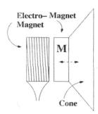
The diagram above shows a very simple loudspeaker. The main part consists of a magnet (mass M) attached to a flexible cone. The speaker is designed so that, in proper use, as the magnet is displaced slightly (left or right) from it's equilibrium position, the cone will push or pull on it with a linear restoring force.
