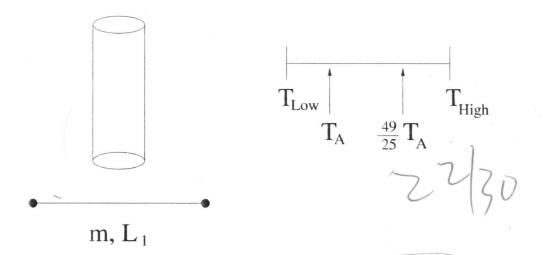
In the apparatus shown, the string (fixed at both ends and driven in its fundamental mode) is used to search for resonant frequencies in the neighboring tube. As the tension in the string is varied from  $T_{low}$  to  $T_{high}$ , the tube is found to resonate at precisely two settings:  $T_A$  and  $\frac{49}{25}T_A$ . For the following, you may assume that the string has a mass m and length  $L_1$ , and you may take the speed of sound in air to be  $v_{snd}$ ...
