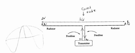
A dipole antenna usually consists of two long horizontal radiating elements that are connected back to a transmitter by means of a feedline. Electrical current flows into and out of the radiators at the points where they are connected to the feedline. Electrical current has to stop at the outer end of each radiator, as there is no place for it to go.
