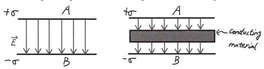
The absolute value of the potential difference decreases since the electric field on either side of the slab stays the same but is 0 inside the slab. Since potential difference is inversely related to capacitance by C: Q, the capacitance must increase.
