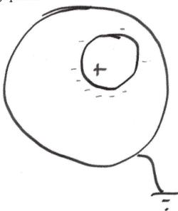
Since the conductor is grounded, no charges will live on the external surface. To balance the positive point charge tq, the total charge on the conducting sphere will be -q. As a result, the electric field will be 0 inside, which is true of all conductors.
