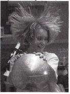
When the kid touches the Van der Graaf generator, the charges lying on its surface are transfered to the kid. This charge builds up in the kids hair, causing the individual follicles to repel one another and maximize the distance between them, which can be seen by them standing on end. If the kid did not stand on an insulator, charge would not have been able to build up on her body, and her hair would not have stood on end.
