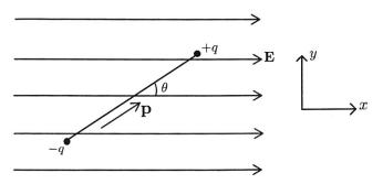
(a) What is the magnitude of the dipole's angular velocity  $d\theta/dt$  when it is pointing along the x axis (i.e.,  $\theta=0$ )? Hint: Use conservation of energy and notice that the electrostatic energy of the dipole in a uniform electric field is  $U=-qDE\cdot\cos\theta$ .
