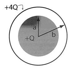
The conducting wire will cause charge to flow from higher potential to lower potential. So the electric potential on the sphere and the spherical shell are equal.
