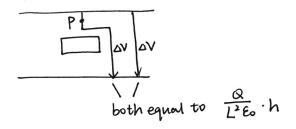
(c) What is the capacitance of the two plates with the dielectric block present? (Hint: you can ignore "fringing" fields; that is you can assume the electric field retains planar symmetry even with the dielectric block present).
