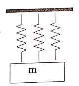
(b) Three identical springs with k=60 N/m are connected to the mass m=1 kg as shown as shown in the figure. The horizontal bar is massless. What is the period of small oscillations?
