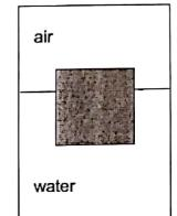
(b) What is the total force F of pressure acting on the bottom of the block, including the atmospheric pressure ( $p_0 = 1.01 \times 10^5 \, \text{Pa}$ ) and the contribution from the water?
