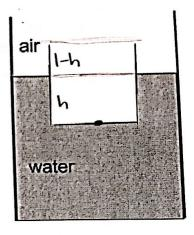
(b) What is the total force F of pressure acting on the bottom of the box, including the atmospheric pressure ( $p_0 = 1.01 \times 10^5 \, \text{Pa}$ ) and the contribution from the water?
