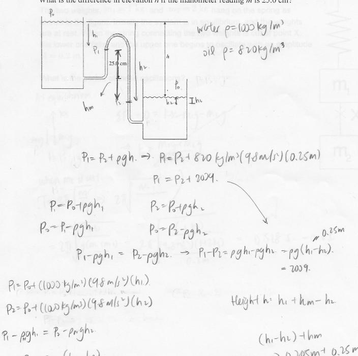
$P_1 - P_2 = p_{mg} (h_1 - h_2)$  $h_1 - h_2 = \frac{p_1 - p_2}{p_{mg}} = \frac{2009}{(wookg/m)(98)} = 0.205 m$   $h = 0.455 \text{m} \times 4.5 \text{ cm}$
