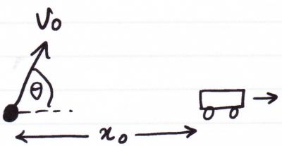
As shown in the diagram a projectile must be launched that it will hit a moving car. You have control over  $\theta$  but  $v_0$  is predetermined. At the time of projectile ( $t=0$ ), the car is a horizontal distance  $x_0$  away from the launch. Car starts from rest and accelerates uniformly at an acceleration of ' $a$ '. Assume that  $v_0$  is sufficiently large that the projectile can indeed hit the car for the given ' $x_0$ ' & ' $a$ '. Find the required  $\theta$ .
