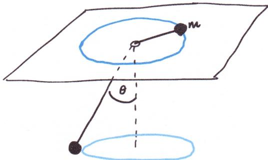
Two point masses each with mass 'm' are connected with a rope with length 'l' which goes through a hole of a horizontal plane as shown. Plane is frictionless. As shown, both are performing circular motion with equal tangential speed.
