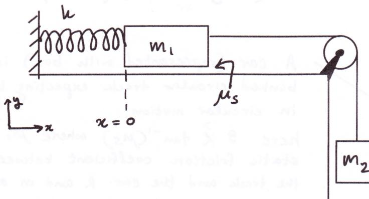
Two boxes with masses  $m_1$  and  $m_2$  are connected with a rope and are setup as shown in the figure.  $\mu_s$  and  $\mu_k$  are static and kinetic frictional coefficient between the box and the horizontal table.  $m_1$  is connected to spring with a spring constant  $k$  which is then connected to a wall as shown. Initially the spring is relaxed. definition of  $x=0$  is shown.
