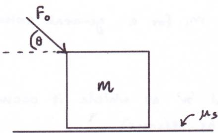
As shown a box with mass  $m$  is sitting on a rough surface where the static friction coefficient between the two surfaces is  $\mu_s$ . An external force  $F_0$  is applied on the box as shown making an angle  $\theta$  with the horizontal.
