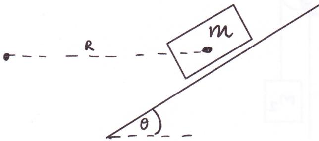
A car (represented with box) is on a banked circular track expecting to drive in circular motion.
