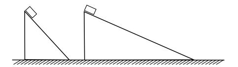
Two identical boxes slide down different ramps pictured above having started at rest from their tops. The boxes start at the same height. The coefficient of kinetic friction  $\mu_k$  between the boxes and the ramps is the same in both cases, and both ramps are fixed to the ground. The coefficient of static friction is not large enough to prevent the blocks from sliding down the ramps.
